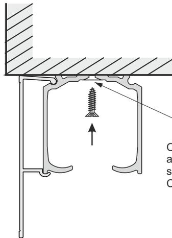
Opening diameters are dependent on screws or bolts used. Countersink screw holes
