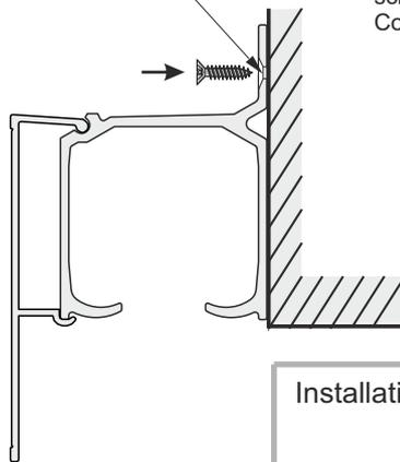
Opening diameters are dependent on screws or bolts used. Countersink screw holes
